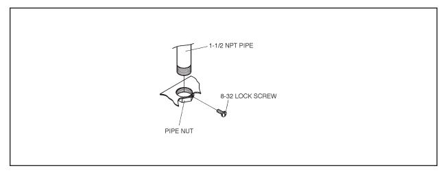
Figure 4. Locking the Pipe Nut
